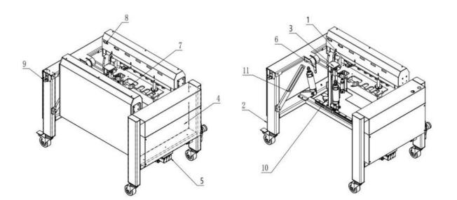
1. Folding side wing parts2. Rack components3. Folded rear wing parts4. Electrical box5. Pneumatic components6. Folding Thousand Wing Parts7. Hitting parts8. Carton clamping mechanism9. Adjust the screw left and right
