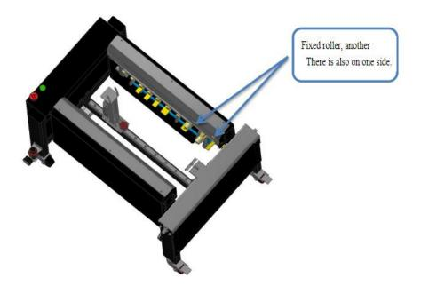
3) Unscrew the plum blossom handle, adjust the front and rear positions according to the length of the box, the total length of the front and rear is longer than the box
