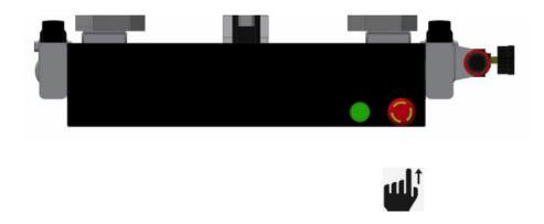
2) Adjust the width of the screw rod, counterclockwise rotation to increase the width, clockwise rotation to decrease the width. Width Slightly larger than the opened width of the box by 2-5mm, to ensure that the box will not be jammed and can be positioned left and right fix.
