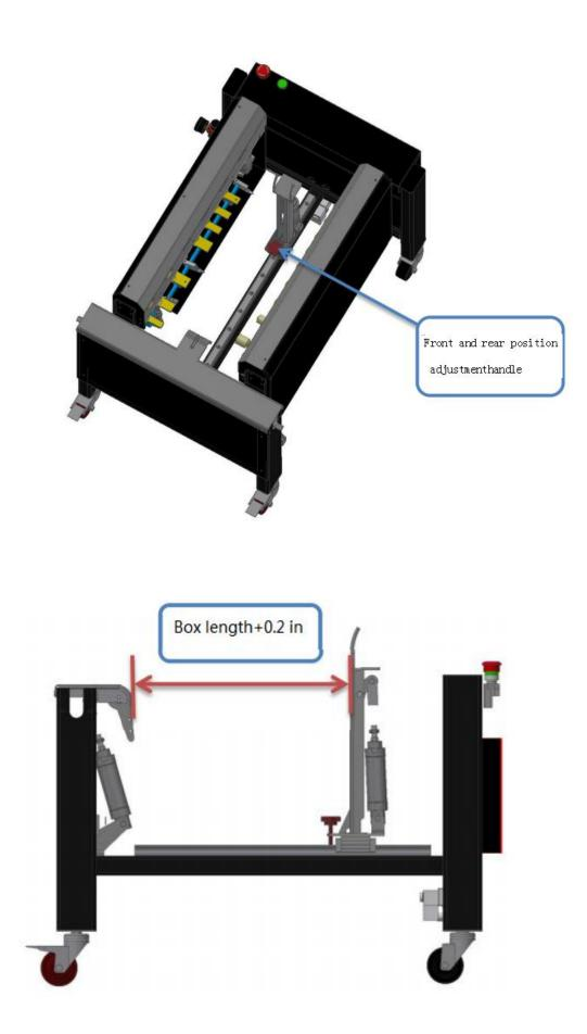
4) Routine adjustment can be ended in the third step. When the box has a large span, the size of the box needs to be suitable
