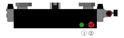
(1). Power switch: start the device after pressing it (provided that the emergency stop button has been unscrewed).
